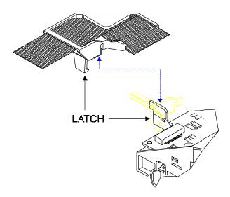
Figure 5-4. Strain Relief Removal/Installation from Carrier.
